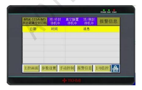
When the equipment is abnormal, the alarm information will be displayed in the alarm information screen, according to the alarm information for alarm processing;
