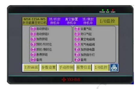
Display PLC input/output point definition, easy to find faults;
