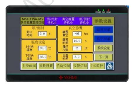
• **Sealing time:** top/side sealing time set value (0~90S), it is recommended to set 5~6s;
